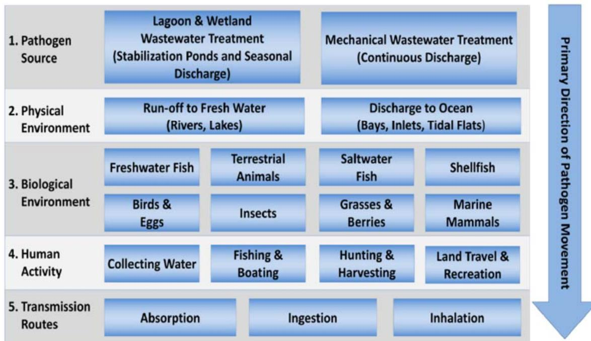
FIGURE 3. POTENTIAL WASTEWATER EFFLUENT EXPOSURE PATHWAYS IN INUIT COMMUNITIES (DALEY ET AL., 2014B).
